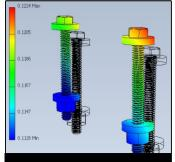
Detailed bolt load calculations for choice of proper anchor arrangements
